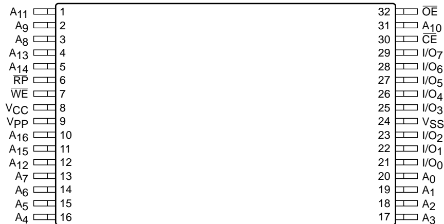
TSOP Package (Standard Pinout) (T, H)
